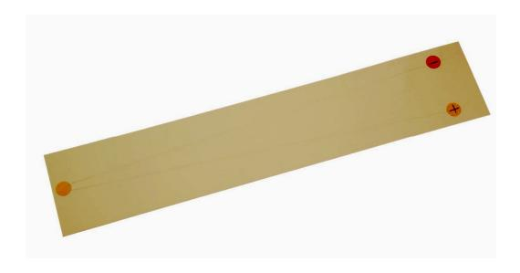
(Illustration shows fine gauge thermocouple mounted to piece of packaging card for protection during transportation)
